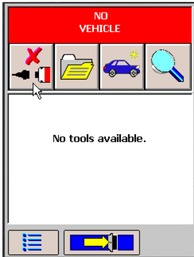
Pic 4: VCM is NOT connected
